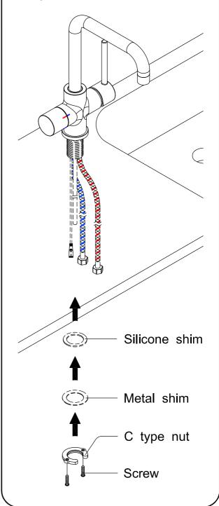
5. Please turn off power supply and water source before piping installation, then connect hot and ambient inlet water metal pipe with hot water source and ambient water source. Connect  $\phi$  8mm drinking water inlet pipe and three way valve to water dispenser as marked in below image. Finally, connect the connection cable with the connector on rear panel, and plug in the power cord.
