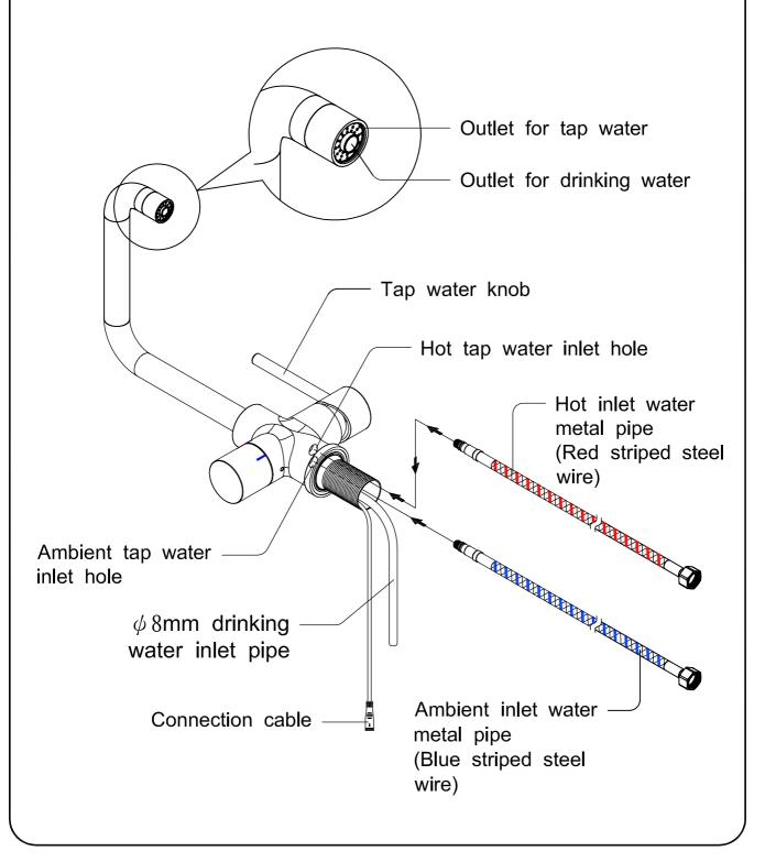
3. After faucet assembled, insert threaded housing into drilled hole including all pipes and the cable.
