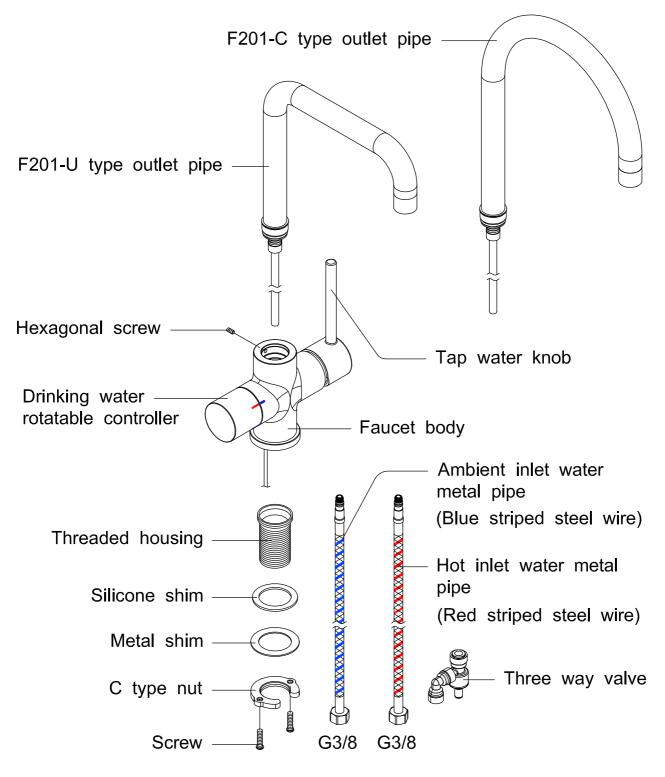
1. Please find the area on the table that is more than 50mm away from the wall, then drill a hole between the  $\,\phi$  32mm to  $\,\phi$  35 mm for faucet installation.
