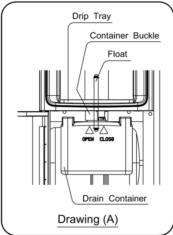
When the float rises higher than the drip tray, as shown in Drawing (A), the drain container is nearly full and must be emptied immediately. The procedures are as follows:
