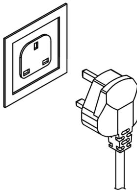
Be sure to use single outlet socket with correct power voltage . Plug the power cord directly into electrical socket .
