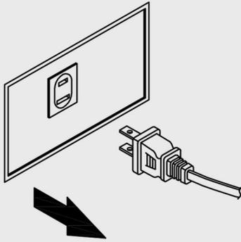
1. Please make sure the machine is completely disconnected from electricity before cleaning.
