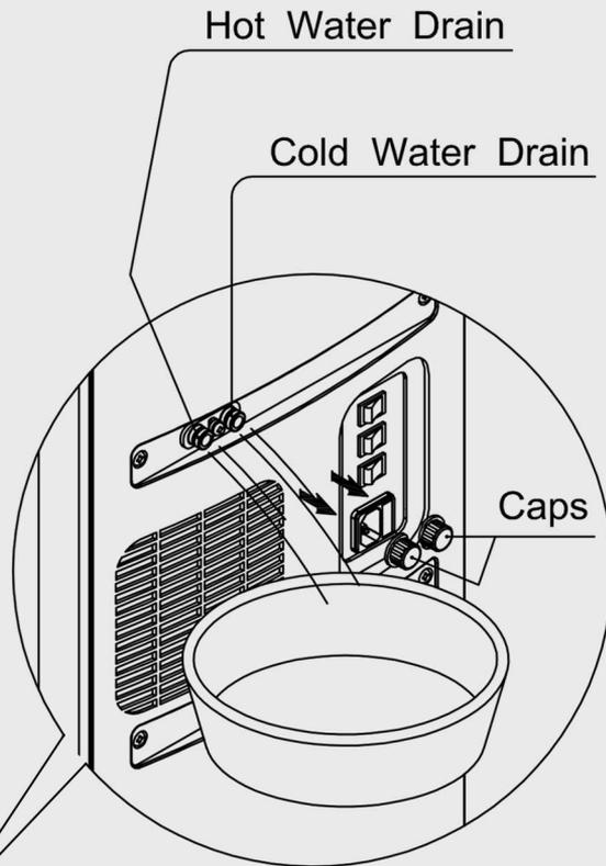
2. Remove the caps on top of the hot water and cold water drains. The remaining water in the tanks will drain out. Cleaning may start when both tanks are emptied. Please put the caps back when cleaning is done.
