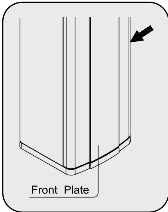
1. Open the lower front plate from the right side as where the arrow is pointing and the container may be seen .
