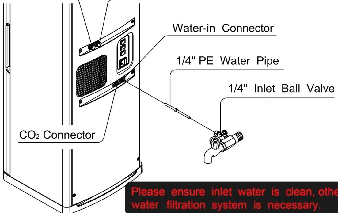
**Please ensure inlet water is clean, otherwise water filtration system is necessary.**
