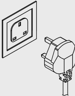
Be sure to use single outlet socket with correct power voltage. Plug the power cord directly into electrical socket .
